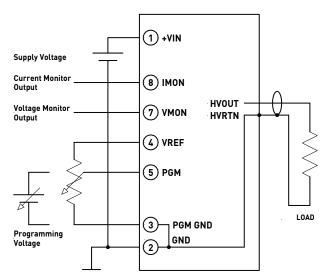
$\label{thm:local_equation} \mbox{High voltage return of the load should be connected to the } \mbox{HV output cable braid.}$
